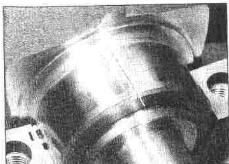
23.7 Plastigage in place on a main bearing journal
