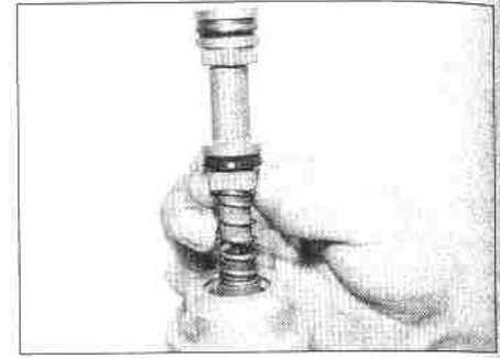
10.14c Fitting the pistons into the master cylinder
