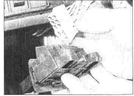
4.4b Disconnecting a column switch multi-plug
