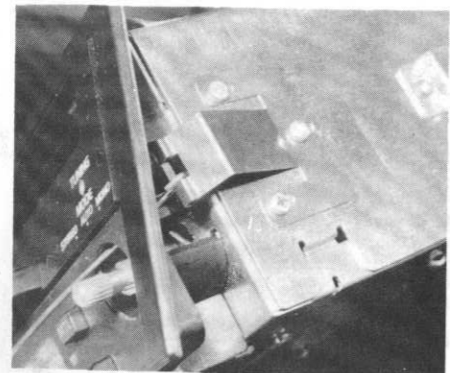
35.4B ... to retract the side clip (unit removed to show clip)
