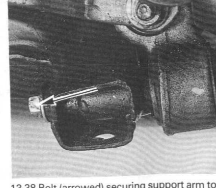
13.38 Bolt (arrowed) securing support arm to hub carrier
