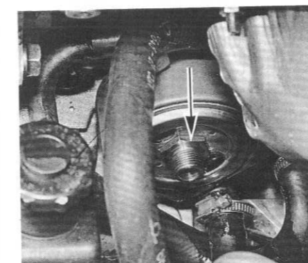
5.24 Oil cooler centre bolt (arrowed)
