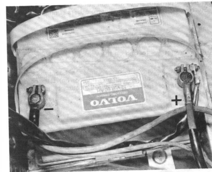
3.1 Battery, showing positive (+) and negative (-) terminals
