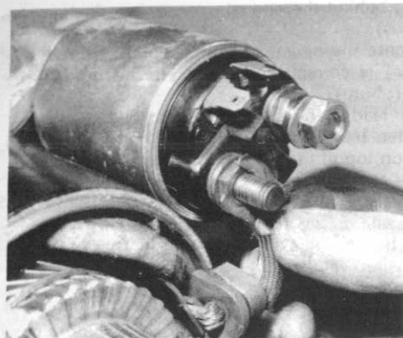
12.21 Reconnecting the motor lead
