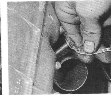
5.15 The earth strap secured by one of the left-hand bolts
