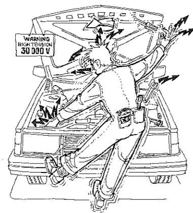
Fig. 4.3 Take care to avoid electric shocks from the HT leads (Sec 1)
