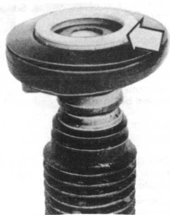
Fig. 13.35 Ball bearing (arrowed) on suspension strut upper mounting (Sec 13)
